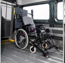
The wheelchair enters the vehicle via lift. AMF-Bruns PROTEKTOR system for wheelchair and occupant restraint.
